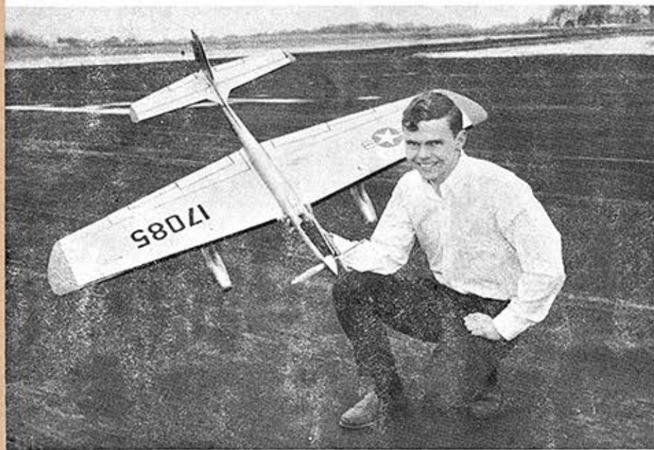
Mike Stott says jet-type stunt jobs attract more attention and get more appearance points. This fully sheeted stunt-fighter with jet pods has many unusual features. His Fox 35 is muffled. Likes it that way.
