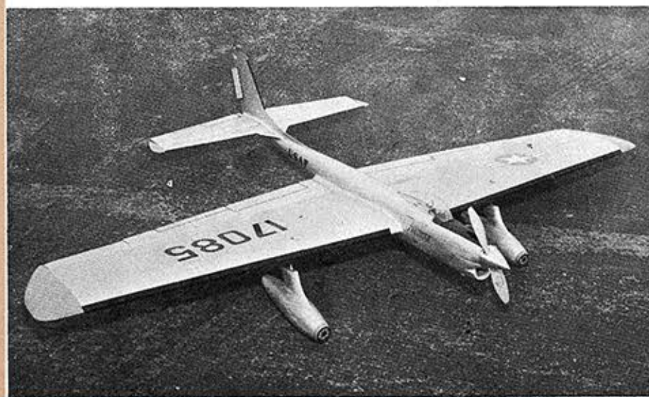
Mike Stott says jet-type stunt jobs attract more attention and get more appearance points. This fully sheeted stunt-fighter with jet pods has many unusual features. His Fox 35 is muffled. Likes it that way.
