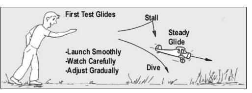
Begin by gliding the model from your hand into a patch of tall grass. Grasp the ship by the fuselage near the balance point, and aim the nose at a spot on the ground about twenty feet in front of you. Launch the ship forward about the way you would a paper dart airplane, nose down.
