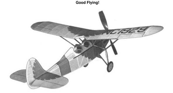
The licence numbers are cut from tissue. Tape tissue to a cardboard backing sheet. Tape the paper pattern on top of the tissue. Cut out numbers with a sharp razor knife and straight edge. Fasten with dope.
