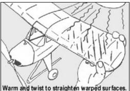
A model can be made to fly with twisted surfaces, but it's confusing to adjust and if the warps change from day to day, you can't detect it. The drawing shows how a surface can be straightened by twisting it in the desired direction while holding it under a heat lamp or other electric heater. Work with it until it is as flat as possible. If your wing has struts, loosen them before bending and re-cement them afterward.
