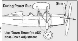
It's not likely that your plane will dive on first power flights, but if it should, put the shim at the bottom of the noseblock, tipping the propeller upward (upthrust).
