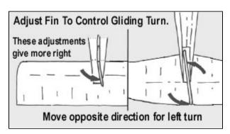
Small changes in fin setting can be made by bending the surface. But if more than 1/32" or so of change is required, cut the fin loose and re-cement it at the desired angle. When the glide is smooth and steady, you are ready to go on to powered tests.
