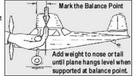
Modeling clay makes handy balancing weight - it can be pressed permanently in any corner. Wire solder or BB shot can be used by cementing in place.
