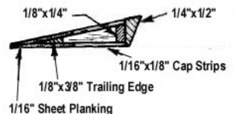
Aileron Rib Cross-Section
