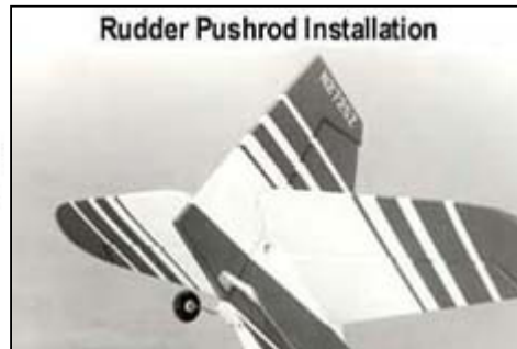
Pushrod Exit Reinforcement Make two from .010 ABS Plastic
