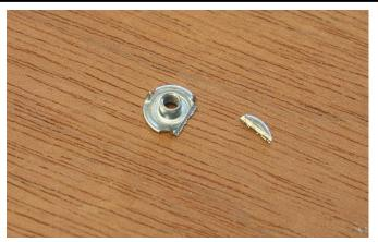
12B...Press the M3 blind nuts into the mount holes in the <u>back</u> of MM-01. Secure them in place with thin C/A Glue. If any of the blind nuts extend past the edge of the opening when the glue is dry, File flush or grind flush with a Dremel tool & sanding drum.
