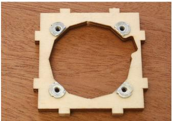
12C...Securely glue the MM-02 / MM-03 assembly to the front of F-7A-EE. Not the orientation of the oval hole in F-7A-EE.
