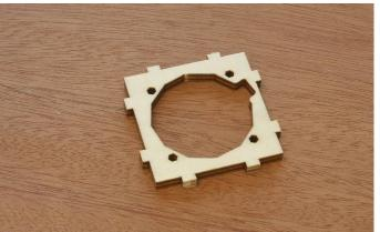
12...Glue parts MM-02 and MM-03 together to make the mount support as shown. Use parts MM-01 and F-7A-EE as a guide to make sure that the assembly is square.
