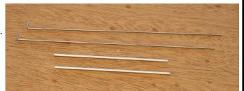
10...Slide the tubes onto the music wire. Position the tube 1/2" from the 90 degree bend and secure the tube to the wire with thin C/A glue.
