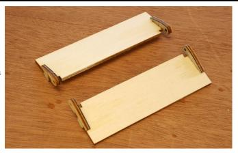
6...Test fit the doors to the bombay. Insert the 2-56 screws and nuts not quite tight.
