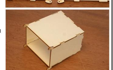
3...Slide B-05 down onto the assembly from the top. The cutouts in B-05 should be at the back end (short end) of the bombay. Make sure that it is seated on top of the legs on the B-02 and B-03 parts. Place part B-04 into place on the top of the bombay.
