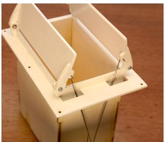
13...With glue or thin servo tape, mount the servo to the top of the bombay in the position shown. Install an EZ connector on the servo arm. Bent the top end of the pushrods as shown and insert them into the EZ connector.
