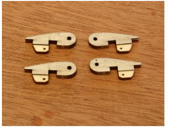
5...Glue the B-07 / B-08 hinges to the B-06 doors. The B-07 on the hinges face inboard...face each other as shown.
