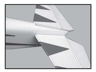
7) After the epoxy has fully cured, remove the masking tape or T-pins used to hold the stabilizer in place. Carefully inspect the glue joints. Use more epoxy to fill in any gaps that may exist that were not filled previously and clean up the excess using a paper towel and rubbing alcohol.
