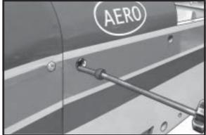
! 4) Install the cross braces. Secure the rear of braces using socket head bolts (type B).
