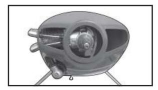
! 3) Install the muffler and muffler extension onto the engine and make the cutout in the cowl for muffler clearance. Connect the fuel and pressure lines to the carburetor, muffler and fuel filler valve. Secure the cowl to fuselage using the 3mmx10mm screws (4).
