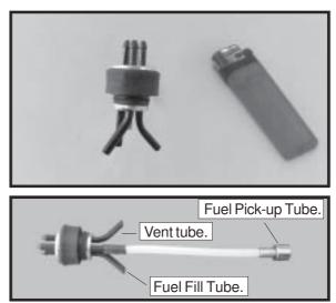
Carefully use a lighter or heat gun to permenently set the angle of the vent tube.
