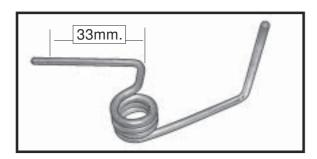
! 1) You have to trim each axles and using a tool cutting and cut-off wheel.
