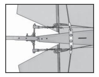
! 4) Secure the tail wheel bracket in place using two 3x25mm wood screws. Be careful not to overtighten the screws.
