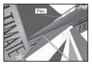
! 4) Remove the stabilizer. Using a modeling knife, remove the covering from below the lines you drew. Also remove the covering from the bottom edge of the stabilizer and the bottom and top edges of the filler block. Leave the covering in place on the sides of the filler block.
