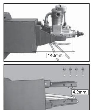
5) Bolt the engine to the engine mount using the four machine screws. Double check that all the screws are tight before proceeding.
