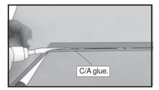
! 6) Using C/A remover/debonder and a paper towel, remove any excess C/A glue that may have accumulated on the wing or in the aileron hinge area.
