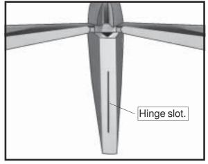
! 2) Slide the vertical stabilizer into the slot in the top of the fuselage. The rear edge of the stabilizer should be flush with the rear edge of the fuselage and the lower rudder hinge should engage the precut hinge slot in the lower fuselage. The bottom edge of the stabilizer should also be firmly pushed against the top of the horizontal stabilizer.
