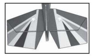
! 8) After the epoxy has fully cured, remove the masking tape or T-pins used to hold the stabilizer in place. Carefully inspect the glue joints. Use more epoxy to fill in any gaps that may exist that were not filled previously and clean up the excess using a paper towel and rubbing alcohol.
