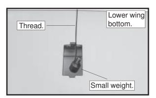
Attach the string to the servo lead and carefully thread it though the wing. Once you have thread the lead throught the wing, remove the string so it can use for the other servo lead. Tape the servo lead to the wing to prevent it from falling back into the wing.
