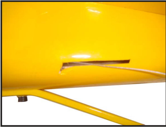
TAILWHEEL PUSHROD HORN INSTALLATION.
