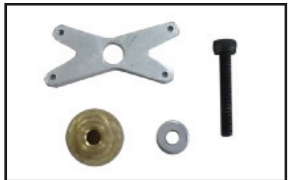
4) Install water rudder control bellcrank to fuselage .
