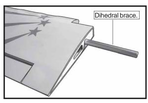
□ 3) Carefully slide the two wing halves together and firmly press them together.
