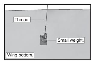
Attach the thread to the servo lead and carefully thread it though the wing.
