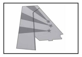
☐ 2) Slide the vertical stabilizer back in place. Using a triangle, check to ensure that the vertical stabilizer is aligned 90° to the horizontal stabilizer.
