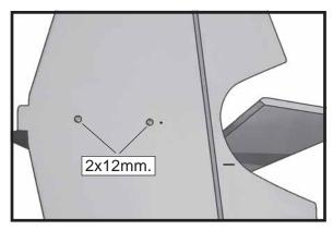
□ 3) Slide the set of vertical and horizontal tail fin to the fuselage.
