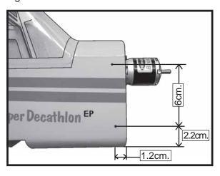
☐ 2) Slide the fiberglass cowl over the engine and line up the back edge of the cowl with the marks you made on the fuselage then trim and cut.
