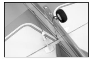
The rudder pushrod is now connected to the rudder control horn, using the same method just used for the elevator pushrod.
