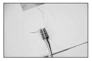
Once the lead is out of the center hole, remove the string from the connector. Leave a little slack in the lead and tape it temporarily to the top of the wing. Turn the wing over and carefully position each servo into its opening in the bottom of the wing.
