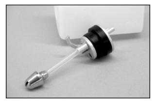
Insert the tank stopper completely into the neck of the tank body. Use a screwdriver to firmly tighten the assembly in place into the tank. Tightening the clamping bolt compresses the rubber stopper, forming a tight seal. The fuel tank is now complete and ready for installation.
