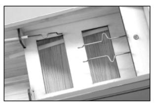
The rudder, elevator, and throttle servos are now installed onto the fuselage servo tray, as shown. We installed the rear rudder and elevator servos first and the throttle servo last. We also found it helpful to first label the servo connectors for later identification when connecting them to the receiver. As shown, position each servo's output arm to approximately line-up with the appropriate pushrod. Install the servos using the mounting screws that came with them.
