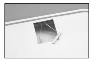
Once the string is loose, remove the scrap balsa piece. Carefully tie and tape the aileron servo lead to the end of the string.
