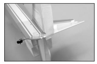
in position to the opposite side, against the elevators. As before, apply 3 or 4 drops of thin CA glue to each exposed hinge edge. Remove the tape and return the rudder to its neutral position. Allow about 10 minutes for the glue to fully wick its way through the surface of each hinge. Flex the rudder firmly in both directions to free up its movement.
