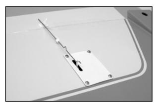
c) Hold the pushrod end against the control horn, at its outermost hole location. Use a fine tipped marker to mark the pushrod wire at the control horn hole location.
