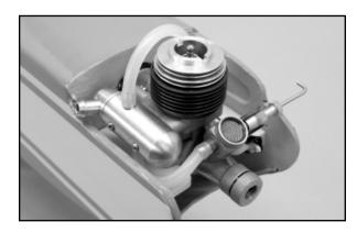
Re-install the output arm retaining screw in the throttle servo. Reassemble the muffler and needle valve back onto the engine. Trim the silicon fuel tubes to fit onto the carburetor and muffler pressure nipple. Be sure to leave enough slack to easily grip these tubes for fueling purposes.
