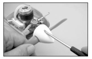
□ 5) The Norvel<sup>™</sup> .074 engine has an exhaust outlet that can be positioned to any desired angle. We positioned ours to aim the exhaust directly out of the right side of the fuselage and then added a short length of large diameter fuel tubing to carry the exhaust past the fuselage side. In actual practice, this works quite well in keeping much of the exhaust residue off the model.
