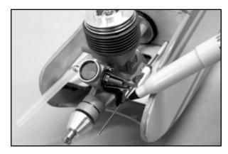
Use a pair of needle nose pliers to make a  $90^{\circ}$  bend in the pushrod wire, at the mark just made. Trim the bent end of the wire to about 3/16". Slip the bent end into the bottom hole in the throttle lever and slide the pushrod retainer forward. Lift the retainer arm over the end of the pushrod wire and press it in place.
